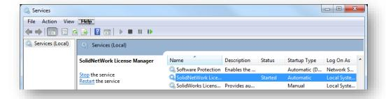
The SolidWorks SolidNetworks License Manager is operational. The next step is to install DraftSight on the client machine. (See point 8, page 21 of this document)
