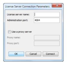
10. Enter the name of the license server (the name of the machine hosting the server, typically). Note that the letters you type are displayed in red until the machine name is found. Then, set the listening port number for the License Administration Tool and click OK.
