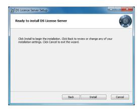
Click the Install button to install the DS License Server. If prompted by UAC to confirm, click the Yes button. The Installing DS License Server dialog box appears, and the progress bar will be displayed. Once the installation has been completed, the following dialog box appears:
